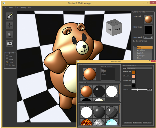
Fig. 4. The interactive 2.5D modeling tool interfaces: In the back, the main window with a Phong shaded shape; In the front, the shading and material library window. Extracted from [10]
